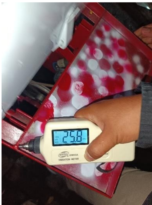
Pengukuran Axial Titik Drive End ( Velocity )
