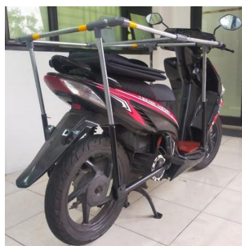
Gambar 4. Sepeda motor listrik sistem hybrid off grid
