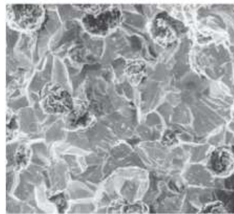
Gambar 2. 6 Hasil Scan Elektron Patahan Brittle Sumber : (Widyanto, 2018)
