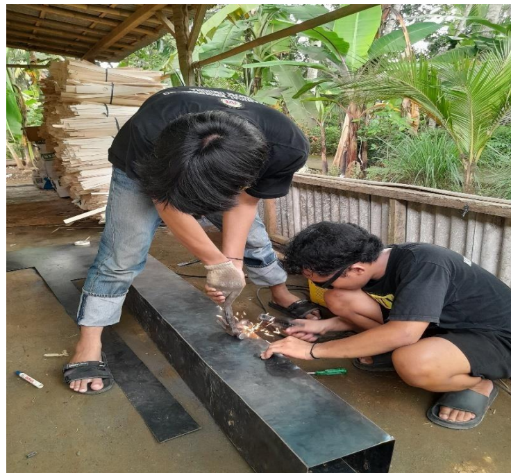
Lampiran 1. Proses Pengelasan Plat Besi
